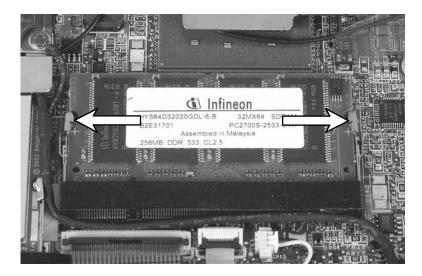
**2** Pull the memory module out of the slot.
